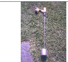
Step 1 - Attach Turf-Tec Cemetery Vase Clean Out Tool to variable speed cordless drill
