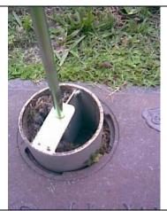
Step 4 -Turn the drill on at a very low RPM and the Cemetery Vase Clean Out Tool removes the debris
