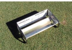
7. Infill depth can also be measured of artificial turf in the same manner to check for uniformity of infill topdressing.
