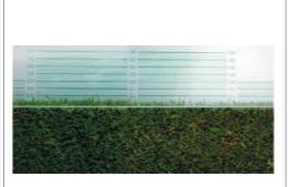
The Grass Height Prism Gauge is made from solid glass and stainless steel. It is designed to tell you the actual height of cut that the mower is making on the turfgrass area. By placing the specially designed prism directly on the golf green, tee, fairway or athletic field and looking through the instrument, you can determine the actual height of cut as well as the quality of cut and smoothness of the surface.
