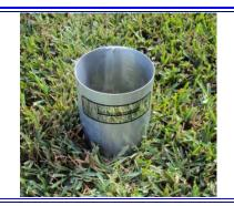
Place the Turf-Tec Insect Flotation Sampler on the area to be tested
