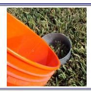
Fill the Turf-Tec Insect Flotation Sampler with soapy water and allow to stand for 3-5 minutes
