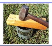
Place a block of wood on top of the Turf-Tec Insect Flotation Sampler and drive it into the soil about 2-4 inched deep
