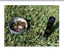
Optional Macroscope 25X shown with the Turf-Tec Insect Flotation Sampler
