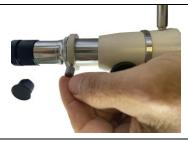
Loosen the depth gauge and adjust downward to prevent lens from touching work surface or object you are viewing
