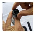
Adjust the eyepiece focus knob (Top of Macroscope) by holding the eyepiece and then turning the focus knob until the inch/mm reticle is as sharp as possible disregarding the image of the object
