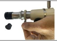
Hand tighten the depth gauge
