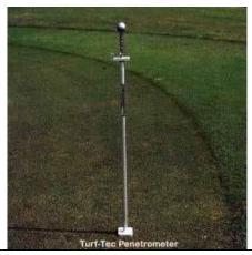
The Turf-Tec Penetrometer is a professional instrument to determine soil compaction.
