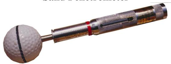
Use the Sand Penetrometer to determine the likelihood of having fried egg lie development in your sand traps. With the easy to use Sand Penetrometer, you can test your bunker sand right on your own golf course to determine if the golf ball will be buried or sit up and be playable.
