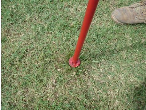
Insert Turf-Tec WeedAway into weeds center
