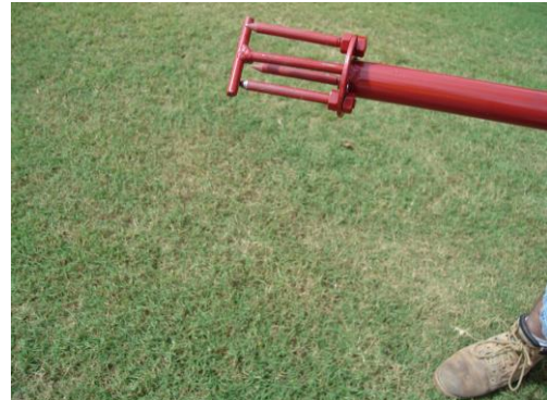
Push sown spring loaded ejection rod to remove weed from tool
