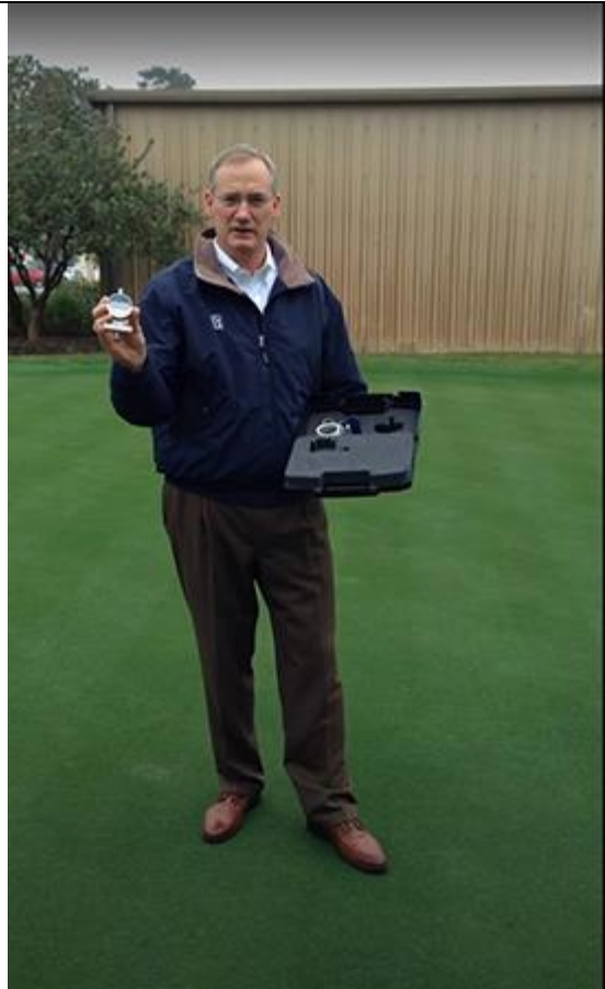
Precision Putting Green Firmness Compaction Meter has a digital depth meter for measuring the depression made in the putting surface after you drop the large bearing
