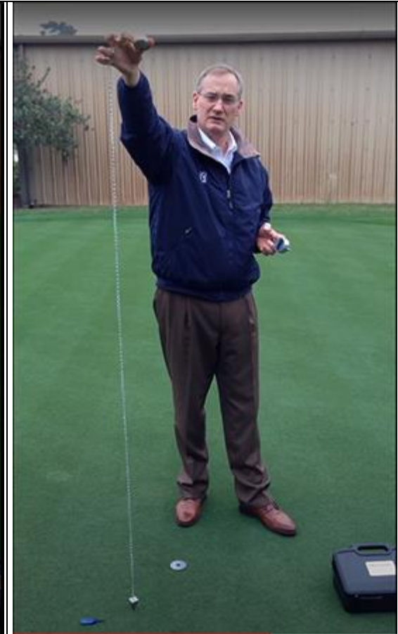
Next, put the six foot measuring chain of the Precision Putting Green Firmness Compaction Meter on your ring or middle finger and extend your arm so the tip of the measuring chain's weight lightly touches the putting green's surface
