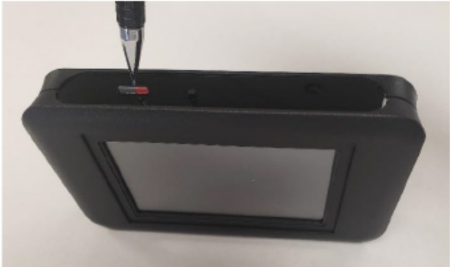
Photo 3 – Using a pen or pointed object, press the SD card in until it clicks. To remove, press SD card in and it will protrude.
