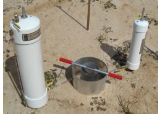
Photo showing IN8P-W Turf-Tec Heavy Duty Tall Infiltration Rings - 6 and 12 inch diameter by 7 inches tall with ports for optional Mariotte Tubes - Ports are located three inches from bottom of rings allowing three inch insertion into the soil and five inches of water on top of soil.
