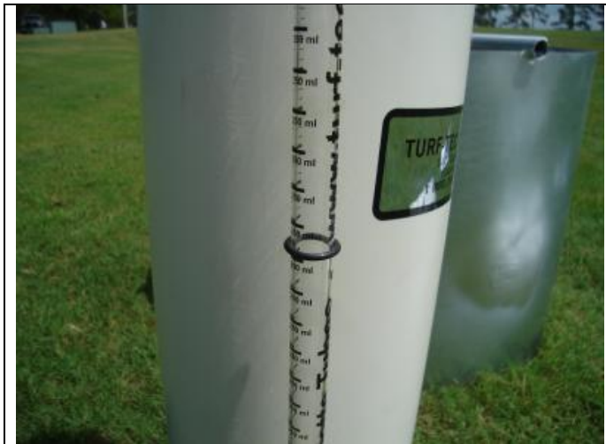
Figure 5 IN12 - Mariotte Tubes water height marker is shown
