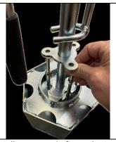
Install screw rods from ejector foot through bottom handle plate. Next install 3 nuts as shown. Finally push screw rods through movable handle plate as shown.
