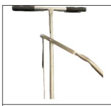
Assemble Cup Cutter Handle to Hex Cutting Head. For mounting PowerStroke™ handle, use the 3 screws that come with the handle, hex bolts & ¼" hex nuts that come with the Hex Cutting Head.
