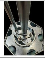
Be sure PowerStroke™ handle is clear from ejector foot screws as shown.
