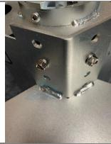
Assemble Footpads to Hex Cutting Head at desired depth by using the 4 (1/4" x ½") hex bolts. Each hole is located at one-inch increments.
