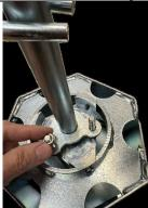
Install 3 nuts on screw rods from ejector foot as shown.
